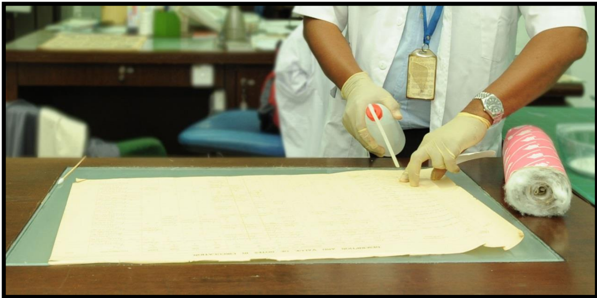
Gambar 7: Ujian kelunturan dakwat
